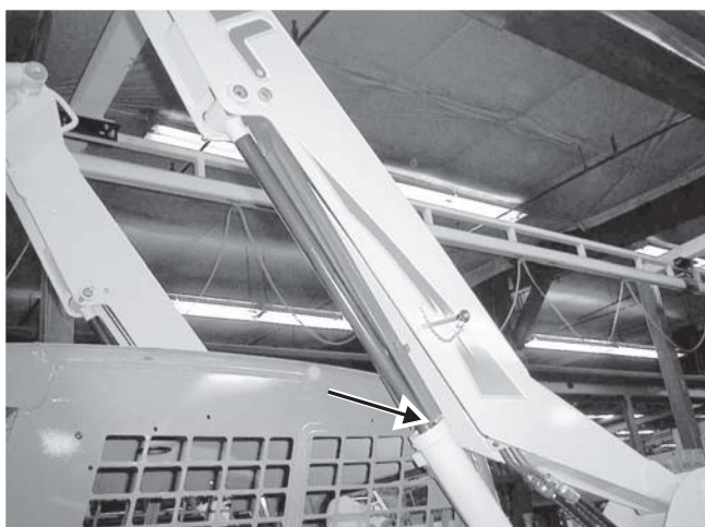
Fig. 2-3 The liftarm support device rests on top of the lift cylinder base.
