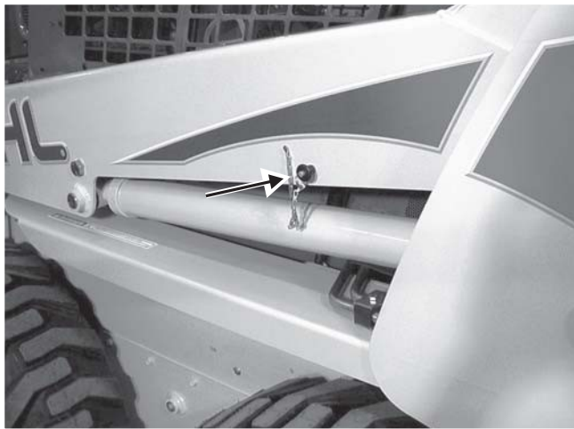
Fig. 2-1 The lock pin secures the liftarm support device inside the left liftarm.
