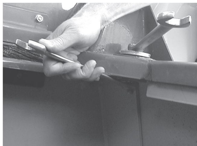
Fig. 2-6 Use wrenches to release the front of the ROPS from the chassis.
