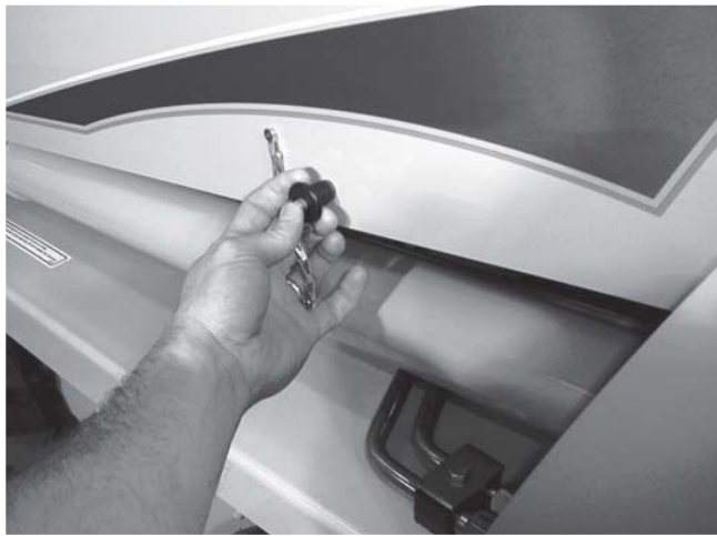
Fig. 2-2 Press in and hold the lock pin button and pull it out.
