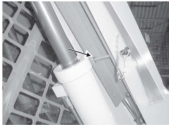
Fig. 2-4 Secure the liftarm support device in its storage position with liftarm fully raised, then lower liftarm.
